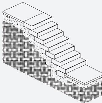
The GRANDE 438 Coping & Step unit is ideal for building stairs with a single unit. Step height is fixed but tread depth can be adjusted by moving the step above forward or backward or by incorporating Navascape pavers in each tread. Due to their size, GRANDE units must be mechanically placed.
