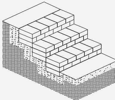
Steps are easily built using a single unit with Antique Hampton Wall. Joints must be staggered for step stability. Cutting of one piece per riser will be required.
