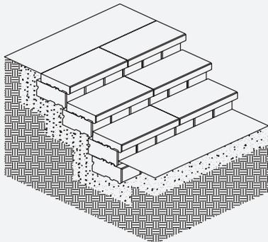
Risers are built using RB Standard units with 10" Coping or 24" Coping units as the tread.
