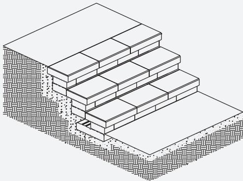
A Double Unit in the base of the bottom riser adds stability. Use 12" Coping units as the stair tread or, for a more comfortable step, Units.
