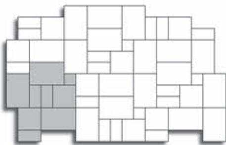
The new Birkdale paver size is optimised to come up with the look of a slab in a 60 mm paver with small chamfer and a smooth finish.
